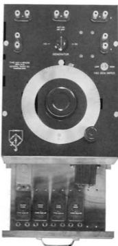
FIGURE 1. The skeleton bridge with the drawer pulled out to show the method of storing standard resistors and condensers when not in use.
