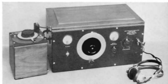
Any pitch between 5 and 10,000 vibrations per second is obtainable from the TYRK 613-B Beat-Frequency Oscillator. Incremental variations on either side of a given frequency are obtained by means of the condenser at the left
